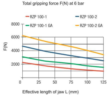
**Type GA/GI with gripping force safety device**
