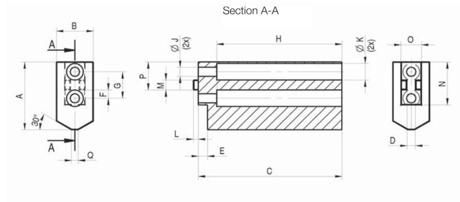
Jaw blank - steel (including fixing screws)
