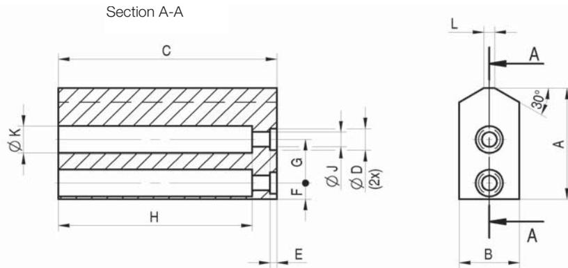
Jaw blank - steel (including fixing screws)
