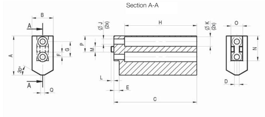
**Jaw blank - steel** (including fixing screws)
