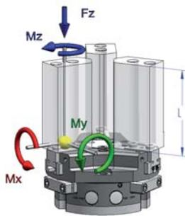
Clamping force diagram exterior gripping
