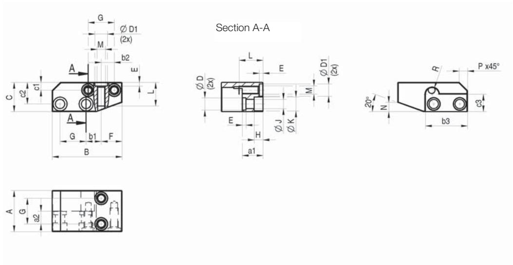
Intermediate jaw - steel (including fixing screws)
