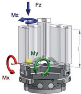
Clamping force diagram exterior gripping
