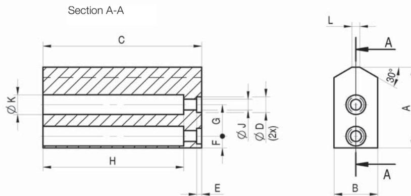
Jaw blank - aluminium (including fixing screws)
